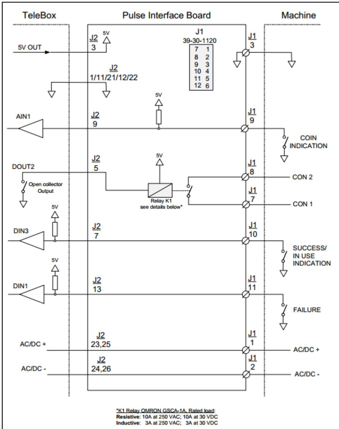
Figure 6 - Pulse Interface board connection schema
