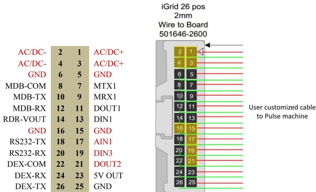
Figure 4 – TeleBox iGrid connector P2 pins
