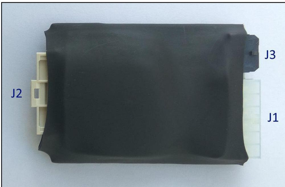
**Figure 8 - Pulse Interface board connectors**
