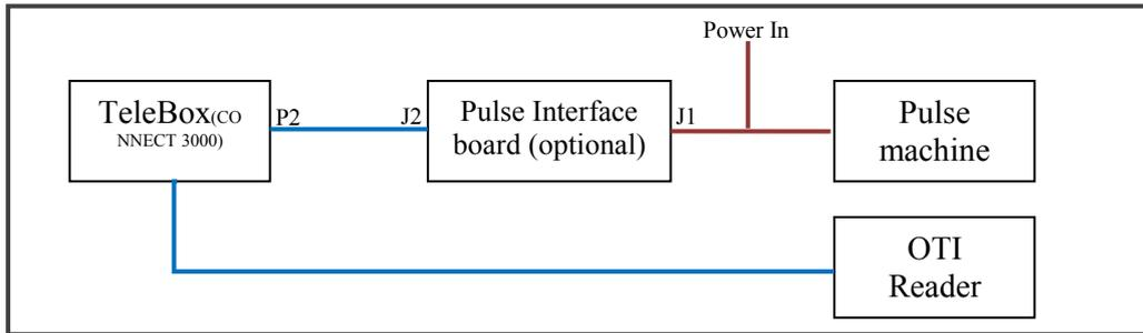
Figure 1 - High level Connection chart
